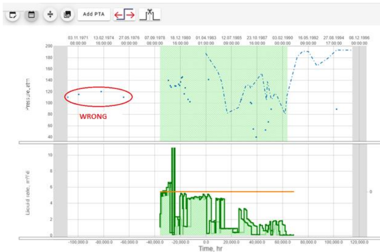
Fig. 1.1.2 – Example of erroneous data with bottomhole pressure readings preceding flow rate values
